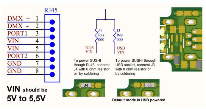
How to use the 2 contacts inputs: make a contact between the Port (pin 3 or 6) and GND (pin 7 or 8) Port triggering is not available by default (option). Contact us to know the price.
