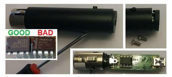
Note: The "DMX chip" is an 8 pin electronic integrated circuit (IC) component located on the electronic card, with the purpose of "driving" the DMX-512 signal.
