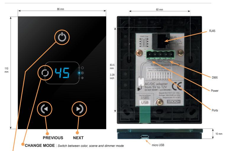
**ON/OFF** : Short touch - Easily switch on and off
